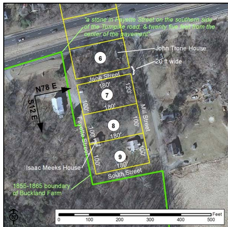
Figure 103: GIS map showing the reconstructed boundaries of Lots 7, 8, and 9 overlaid on recent aerial photography. Boundaries of Buckland Farm ca. 1855-1865 are shown in green and have been rotated 2.1° westward (counterclockwise) to account for historic variation in magnetic declination as estimated by NOAA's National Geophysical Data Center historic declination calculator ( http://www.ngdc.noaa.gov/geomag-web/#ushistoric ).
