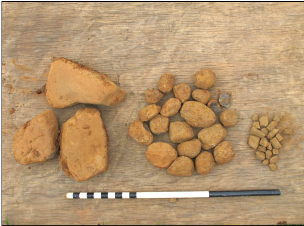
Figure #58: Road metal samples recovered from trench A unit 3 stratum 6 (right), stratum 7 (center) and stratum 8 (left).
