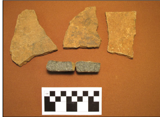
Figure #82: Flat sheets of diabase showing dark gray interior.
